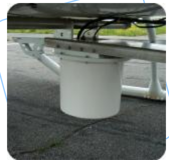
Pod with antenna and integrated GPS
