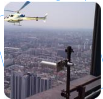
Transmission equipment on a helicopter and a receiving antenna « Diversity » on a building roof.
